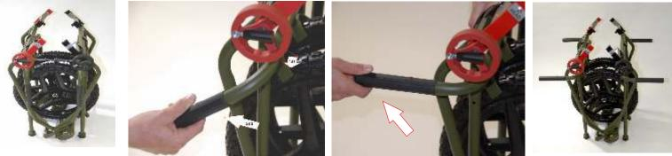
3.) Stand alongside the carrier, grip each side of the unit between the clamps and push the two sides away from each other. Remove the wheels and place them nearby with the pins facing up, clear of debris. Engage the two sides of the carrier by forcefully pushing down until a "click" sound is heard and the two sides are locked in place.
