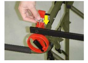
• Once the rail cubes are inserted, slide quick pins into each hole on all four brackets. These will ensure that the brackets stay locked in place.
