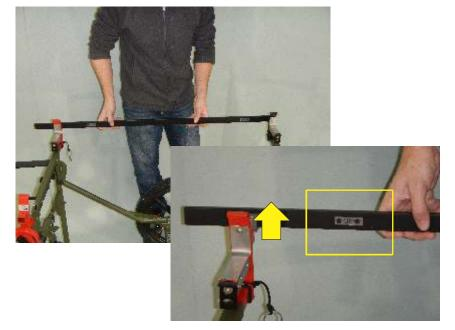
• The accessory rails will only fit if the correct end is pointed toward the RIGHT side of the WLC, while facing it. This end will always be the end with more rail located on the outside of the insertion hole.
